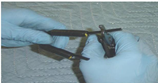
Electrical Tape can be a bad thing and cause the pellets to burn to fast. You only need enough tape to hold them to the line. Prior to Moving
