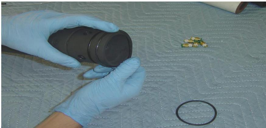
**Step 2:** Begin by installing all O-Rings onto Nozzle and Injector Baffle. All O-rings are Dash Number 230. O-Rings should be free from any cracks, burns or damage.
