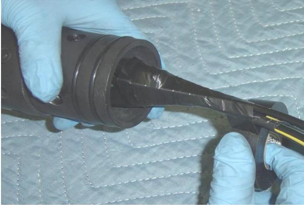
**Step 6:** Using your roll of electrical tape, start taping around all 5 nylon lines. This will slightly pull the lines towards the center of the motor, and ensure the heat of the Pyrodex Pellets at ignition is kept near the lines to ensure a positive ignition. You will only need a single layer of tape over the line set to hold them together.
