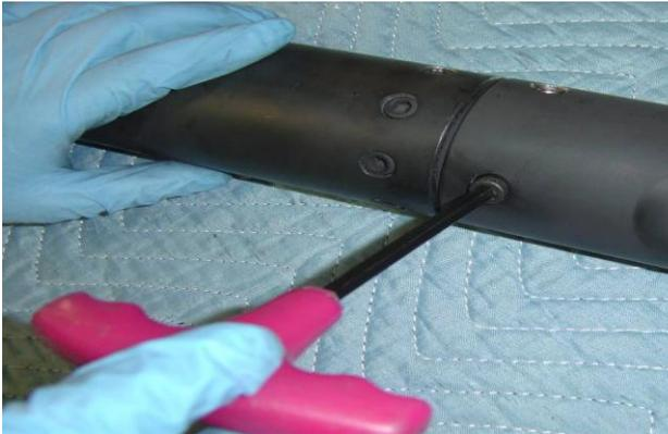
**Step 7:** Grease the Injector Baffle O-rings and slide the nitrous tank section of the motor onto the combustion chamber and insert the retention bolts. The bolts will require a  $\frac{1}{4}$  inch hex head wrench.
