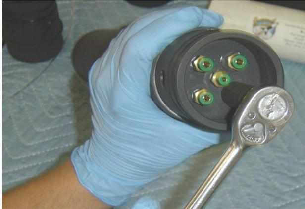
**Step 3:** Insert Press Lock Fittings into the Injector Face. A 1/8 Inch Fitting will always go in the center port. 1/8 inch Fittings are used for Slow Motors, 3/16 for Medium Motors and 1/4 Inch for Fast Motors. The Fittings should be tightened 1/2 turn past tight.
